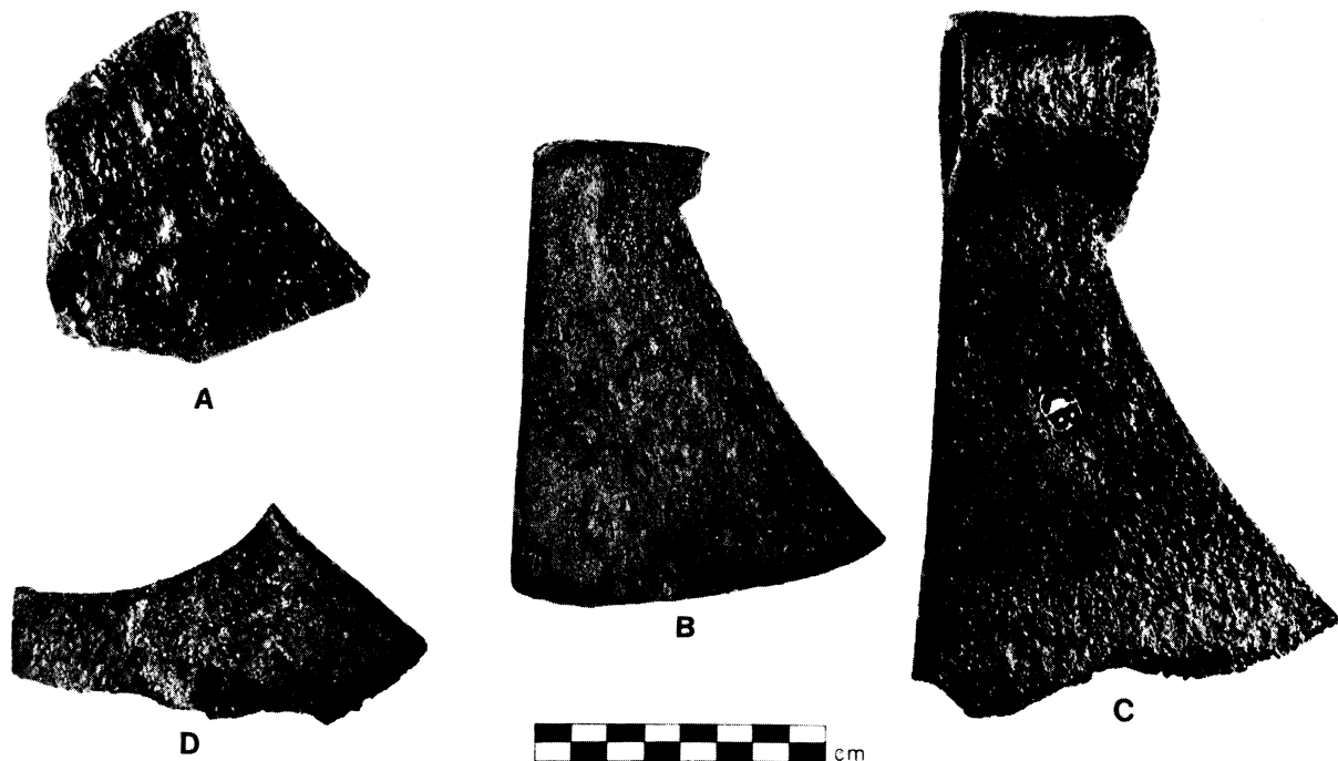
Figure 1. Large trade hatchets. A - (Feature 5) Blade with hammered top. B - (No. 460) Steeled blade with hammered top. C - (No. 16) Complete hatchet with smiths' mark and bent and broken bit. D - (No. 510) Steeled blade broken through "steel" and across wrought iron upper blade.
